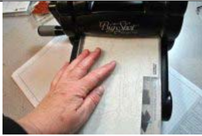
Run the cardstock and folder through on Tab 1 and between two clear plates
